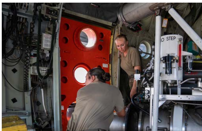
Above and Below: Maintainers from the 152nd Maintenance Group attach the Modular Airborne Fire Fighting System Equipment nozzle onto the left rear door on MAFFS 8 before the aircraft is launched to the Channel Islands Air National Guard Station at Port Hueneme to report for MAFFS activation on July 17th.
