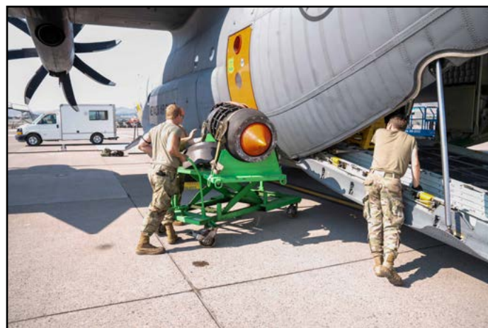
Above and Below: Maintainers from the 152nd Maintenance Group attach the Modular Airborne Fire Fighting System Equipment nozzle onto the left rear door on MAFFS 8 before the aircraft is launched to the Channel Islands Air National Guard Station at Port Hueneme to report for MAFFS activation on July 17th.
